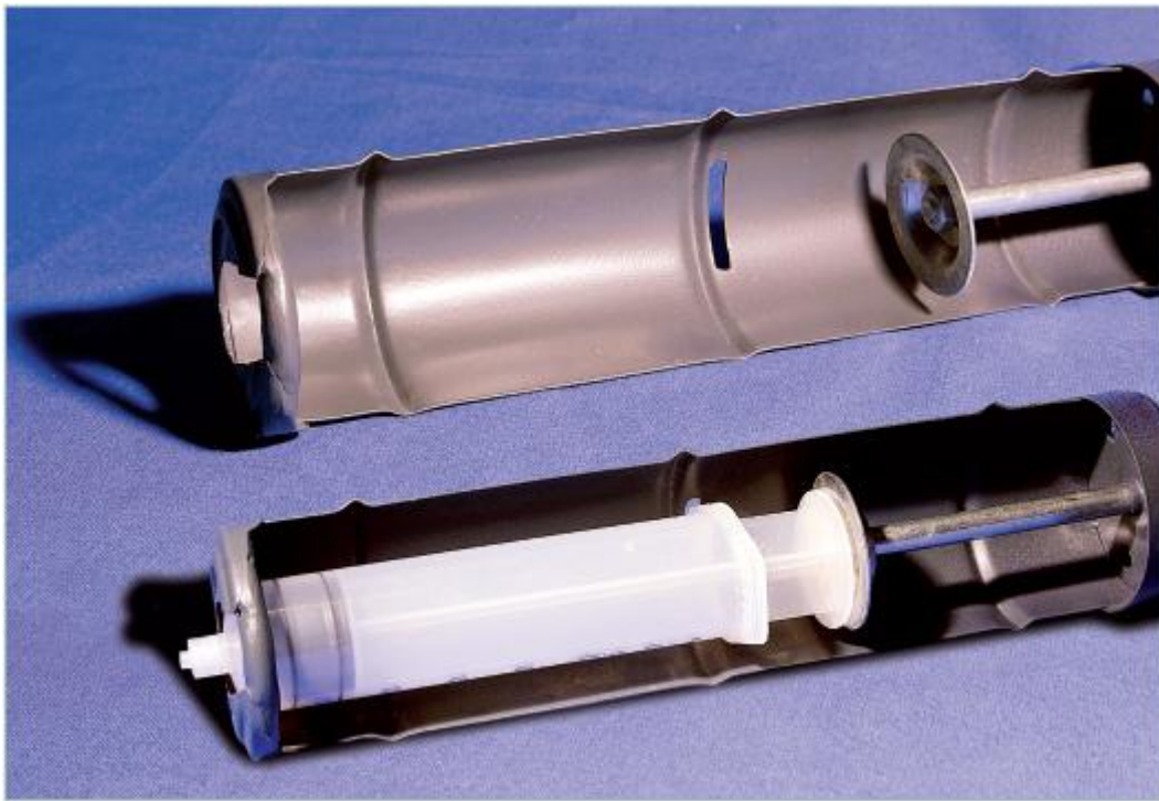
Fig. 8. Professional silicone application gun adapted to hold a 10-50 ml syringe.
